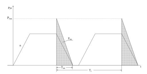
The ohmic value of the normalized resistors has been calculated in order to assure the braking current for the limit use of 6KBU300, that is to say a 460Vac supply of the inverter (braking threshold 745Vdc).
